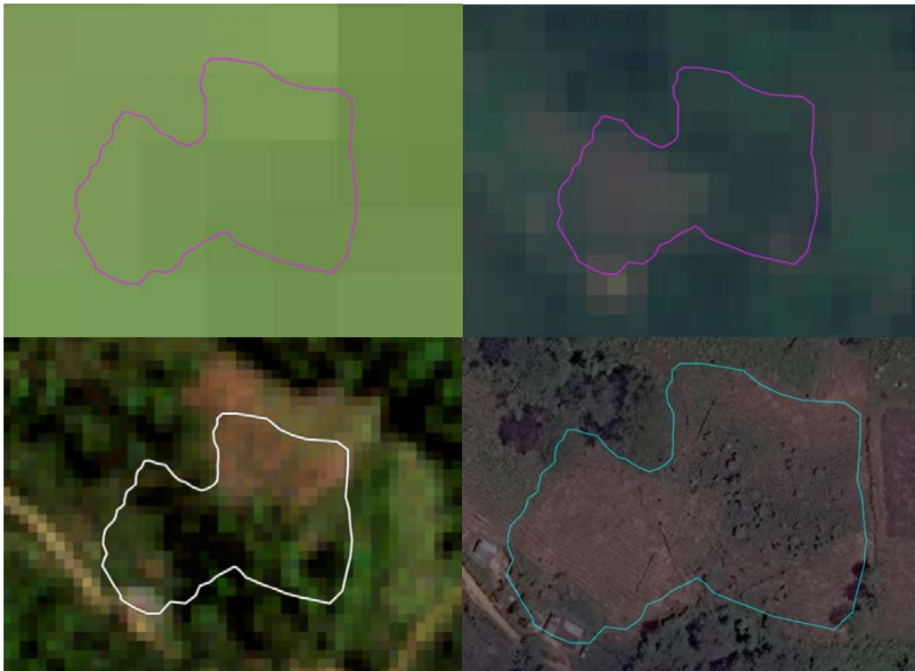
Figure 2.4. Comparison of 30m Landsat imagery (top left), 10m Sentinel 2 imagery (top right), 4m Planetscope imagery (bottom left, Vantor 2025), and 30cm WorldView 3 imagery (bottom right, Vantor 2025).
