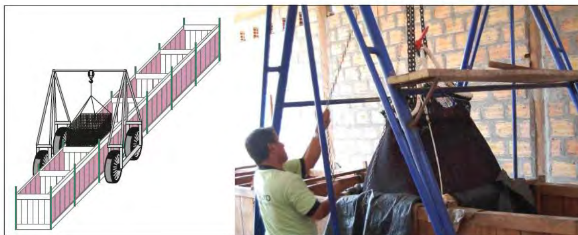
Figure 2 Modern system for fermenting cocoa beans using winch to lift and move beans from box to box. Boxes are flat on floor and one worker can turn beans when ready.
