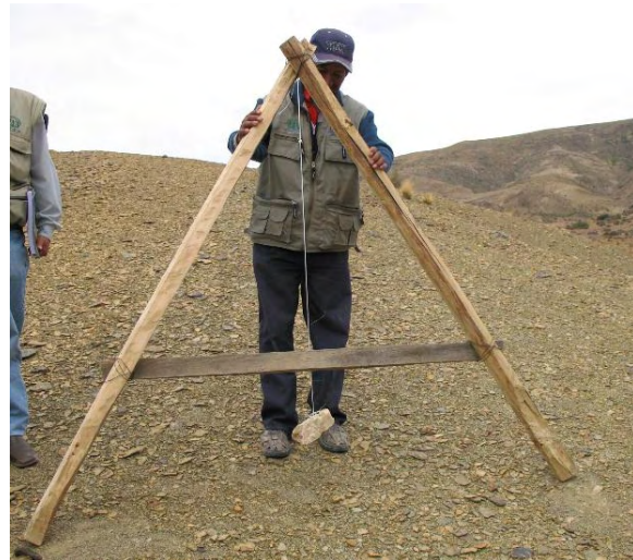
An A-level is made with simple material: poles, wire, string and a stone, but it allows farmers to trace a contour line.
