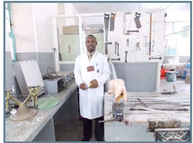
Figure 33. The area in the workshop used for acrylic lamination requires local exhaust ventilation of irritant gases.
