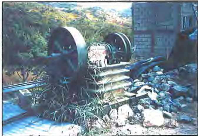
A 80-horsepower crusher made by Universal Crusher Company of Cedar Rapids.
