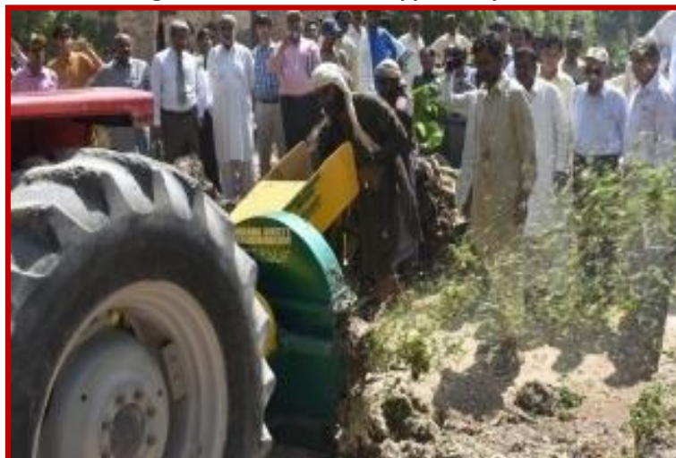
Image 8 Banana Residue Chopper in Operation
