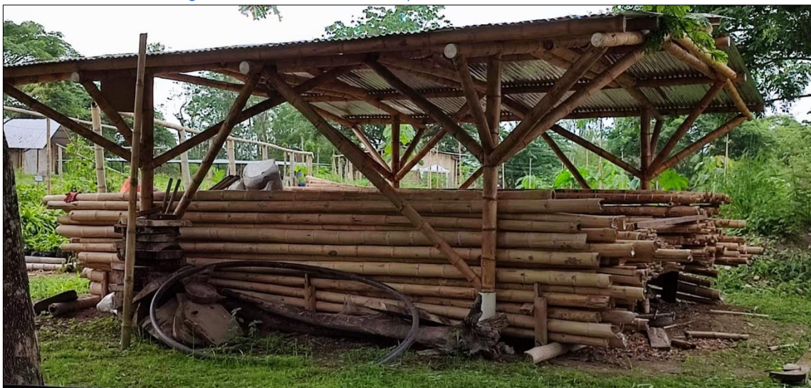
Image 14 Treated guadua cane in the process of drying in the Production Center of the associations of artisans and bamboo builders of the Pedernales canton. ASOPROASE and ACERO VEGETAL
