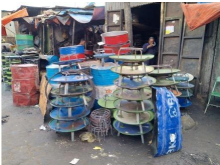
Steel VO cans converted into charcoal grills at Minalesh Tera market, Ethiopia Source: Fasil Reta, 2021
