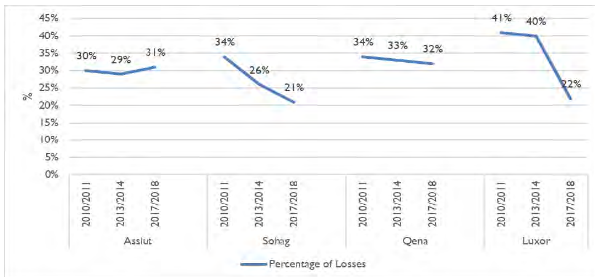
GRAPH 2: PERCENTAGE OF WATER LEAKAGE BY SUBSIDIARY COMPANIES (2010/2011 – 2017/2018)
